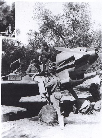
LEFT AND BELOW: These close ups show the Junkers Ju 210 Da twelve-cylinder inverted-Vee liquid cooled in-line engine fitted to the Bf 109 D-1. For many years after the war, it was thought that the D-variant was powered by the experimental 1,000 hp Daimler-Benz DB 600 A engine, a result of successful German propaganda.
