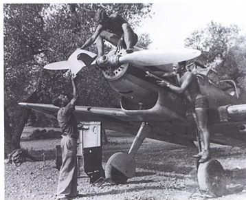
A series of photos showing routine servicing being performed on one of J/88's Bf 109 B-2s. The type was powered by a 600 hp Jumo 210 twelve-cylinder liquid-cooled in-line engine which gave it a maximum speed of 465 km/h (298 mph). The variant also differed from the B-1 in carrying a third 7.9 mm MG 17 machine-gun mounted between the engine cylinder banks, firing through the propeller hub. The first Messerschmitts that went to Spain were not equipped with radio equipment although this became standard in later variants.
