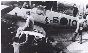
LEFT AND BELOW: Ground crews struggle to recover this Bf 109 E, coded 60107, after the starboard undercarriage leg collapsed. The aircraft has the legend "Mors Mors" painted above the exhaust in white.
