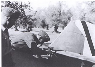
A series of photos showing routine servicing being performed on one of J/88's Bf 109 B-2s. The type was powered by a 600 hp Jumo 210 twelve-cylinder liquid-cooled in-line engine which gave it a maximum speed of 465 km/h (298 mph). The variant also differed from the B-1 in carrying a third 7.9 mm MG 17 machine-gun mounted between the engine cylinder banks, firing through the propeller hub. The first Messerschmitts that went to Spain were not equipped with radio equipment although this became standard in later variants.
