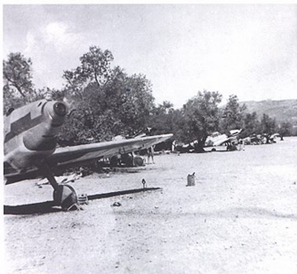
ABOVE: A pair of Bf 109 B-2s in service with Jagdgruppe 88 during the autumn of 1937. The first Messerschmitts were delivered in overall pale grey (65) finish but later this was overpainted with irregular medium green (62) stripes, with the undersides painted in pale blue (65).
