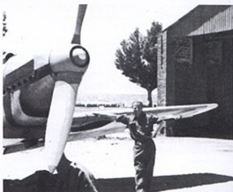
ABOVE: A close-up view of the two bladed wooden propeller as fitted to the Bf 109 B-1.
