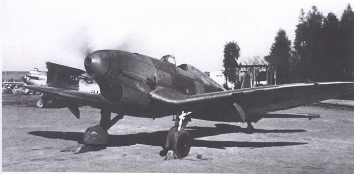
ABOVE: The He 112 V3 arrived in Spain in November 1936 where it was test flown by Oblt. Günther "Fips" Radusch. The prototype, which had been built without armament, had been fitted with an experimental engine-mounted 20 mm C/30 L cannon for tests. Shown here at Tablada airfield, the aircraft was given the code 501 and was later flown operationally against Republican armour by Uffz. Max Schulz of 1./J88 who destroyed three tanks.
