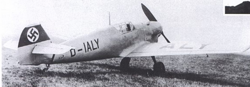
ABOVE: A close-up view of the two bladed wooden propeller as fitted to the Bf 109 B-1.
