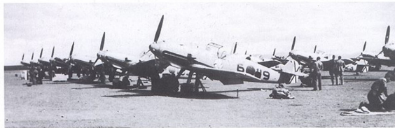
RIGHT: Illustrated in colour above, this Bf 109 E was flown by Siebelt Reents, Staffelführer of 1./J/88. Note the black area painted from the exhaust to behind the wing leading edge designed to hide the smoke blackening from the Daimler-Benz DB 601 engine.
