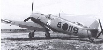
RIGHT: Illustrated in colour above, this Bf 109 E was flown by Siebelt Reents, Staffelführer of 1./J/88. Note the black area painted from the exhaust to behind the wing leading edge designed to hide the smoke blackening from the Daimler-Benz DB 601 engine.
