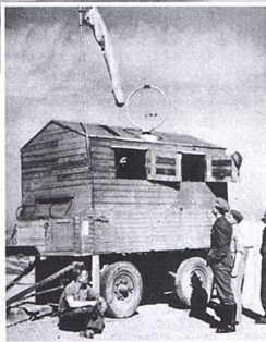
ABOVE: A mobile communications hut which was used by the Legion Condor. From the middle of 1937, radio transmitters/receivers began to be installed in the Bf 109s of J/88 which proved a great advantage. The vehicle, seen here, was basically a "shed on wheels" with a D/F aerial mounted on top and a windsock.
