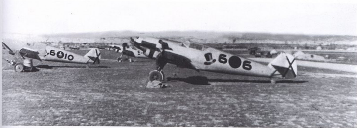
ABOVE: Photographed at Escarón airfield during the Aragón offensive, this group of Bf 109 B-1s carry the later style of marking system, with the aircraft type number forward of the black national insignia circle and the individual number aft. Previously Bf 109s had both numbers painted behind the circle, with a hyphen between. 606 in the foreground was flown by Fw. Herbert Ihlefeld before being written off by Uffz. Franz Jaenisch in July 1938. It has had the wooden propeller replaced by a Hamilton metal unit.
